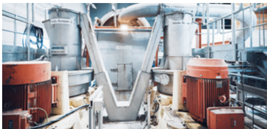
ANDRITZ ModuScreen TD coarse screen as part of the stock preparation plant
