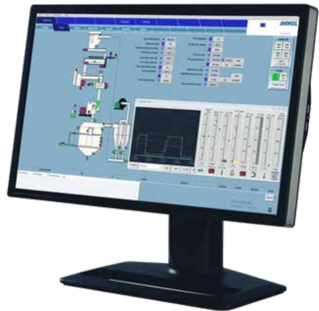
Example of an ANDRITZ ASCADA overview screen with trend popup overlaid
